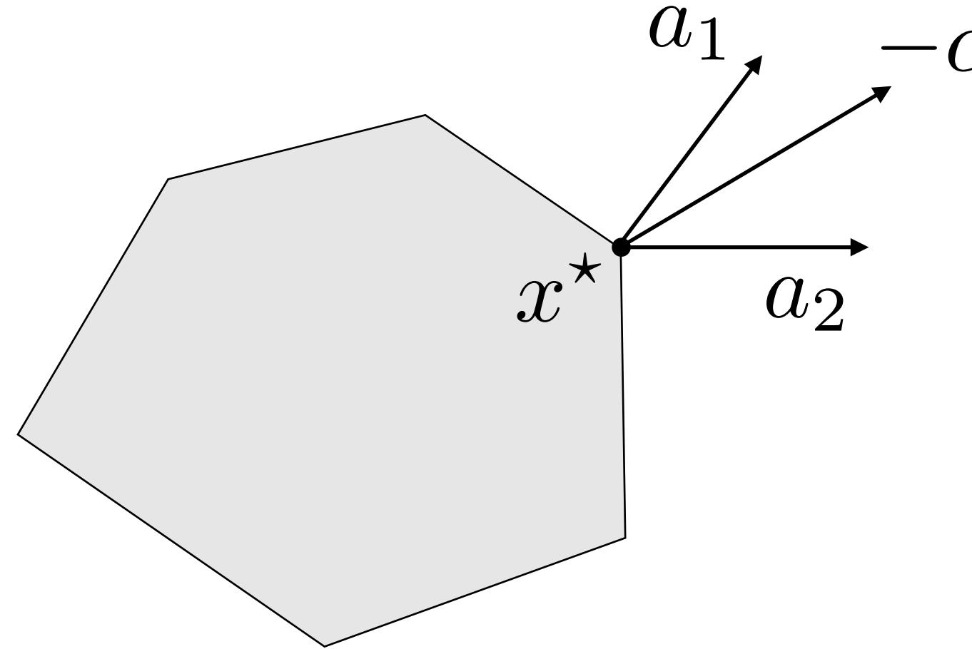
Two active constraints at optimum:  $a_1^T x^* = b_1$ ,  $a_2^T x^* = b_2$
