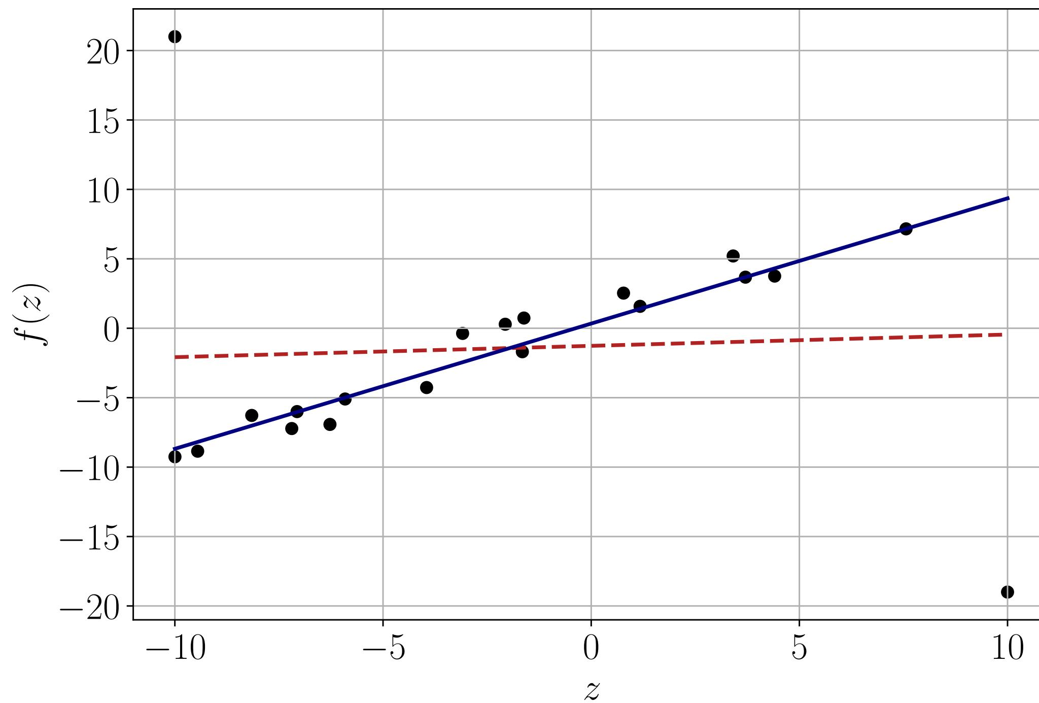
$$\begin{bmatrix} 1 & z_1 \\ \vdots & \vdots \\ 1 & z_m \end{bmatrix} \underbrace{\begin{bmatrix} \underline{a} \\ \underline{b} \end{bmatrix}}_x \approx \begin{bmatrix} f_1 \\ \vdots \\ f_m \end{bmatrix}$$
